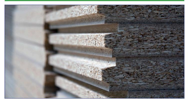
To complement project specific coatings and films, TFS also offer a complete range of machining services, including cut to size, tongue and grooving, routing and sanding. This comprehensive machining and profiling service saves you time and money on site by offering site ready fabrication.
